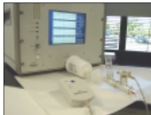
FIGURE 3: MODEL USED FOR MEASURING AEROSOL DELIVERY WITH SIMULATED ADULT BREATHING PATTERN. SHOWN WITH AERONEB PRO WITH DOUBLE ONE-WAY VALVE SYSTEM.
